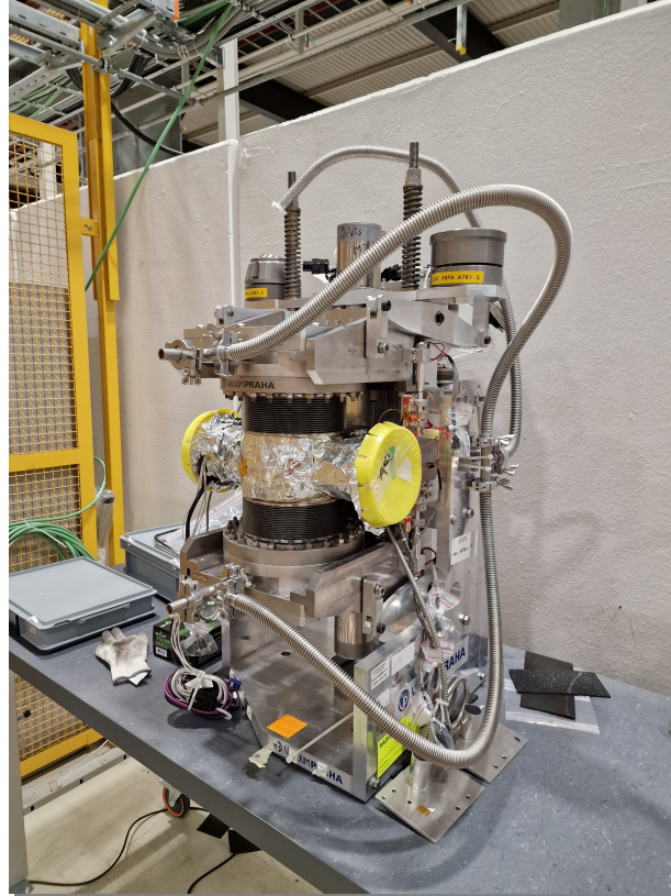
ALFA detectors removed Station refurbishment ongoing
