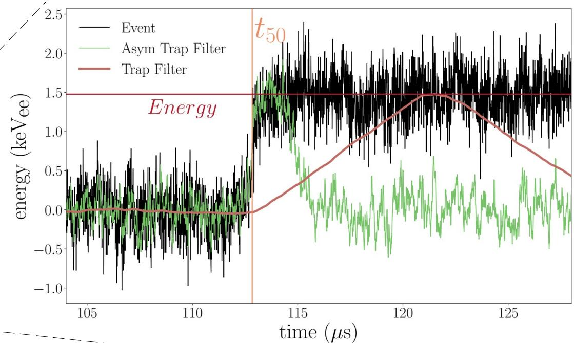
height of step  $\sim$  energy of particle
