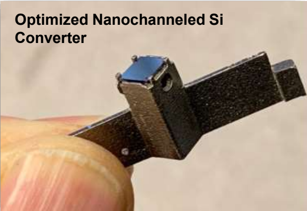
on-axis miniature Ps formation target
