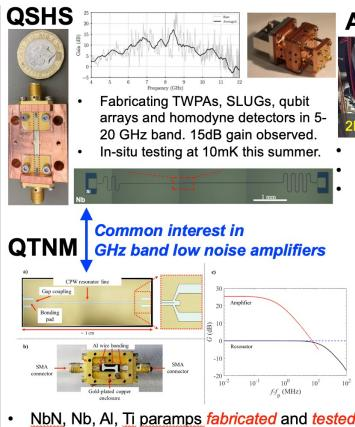
at 18 GHz for QTNM . Operation at ~100mK
