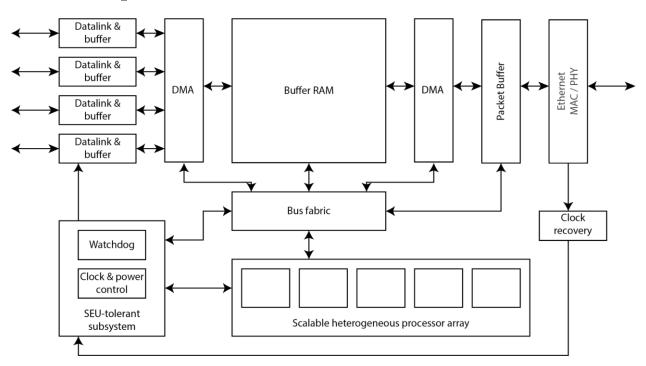
Proposed common interface ASIC for detector readout, timing, & control
