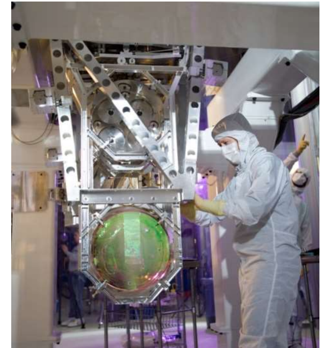
aLIGO QUAD suspension (3/4 stages of vertical/horizontal isolation)
