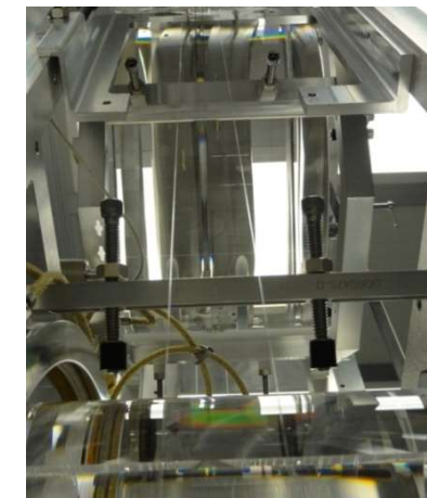
Final mirror suspended by fused silica fibres (Q factor >10^9 )
