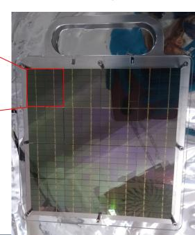
Signal readout is 1 channel per 4 tiles -> 4 channels per PDU.
