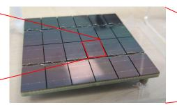
Photo Detection Units (PDUs) are 20 x 20 cm SiPM arrays consisting of 16 tiles.
