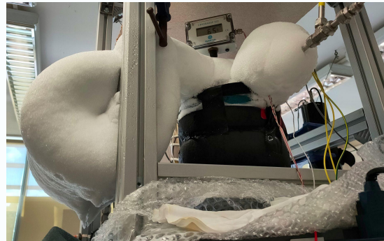
Above the STEEL dewar; the steel coil acts as a nucleation point for frost build-up
