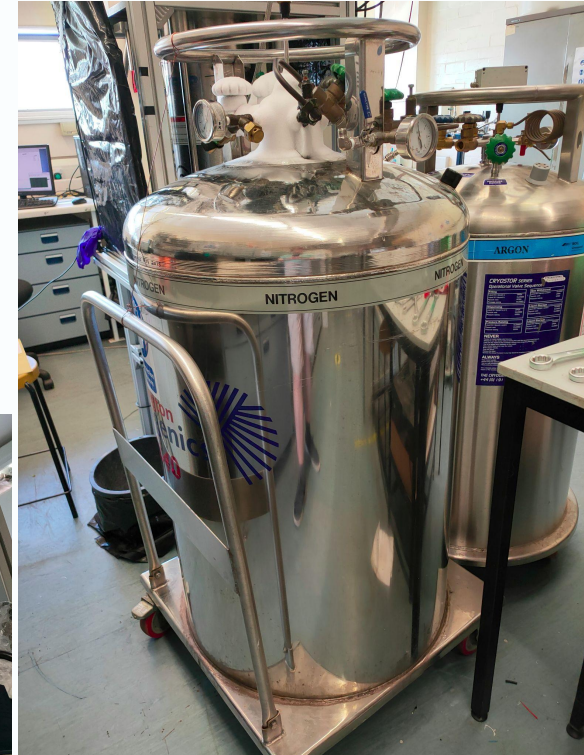
40 l LN (left) and LAr (right) cryogenic containers, filling the STEEL condenser and dewar respectively.
