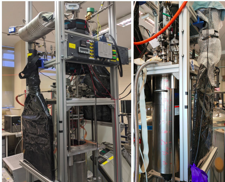
Photos of STEEL with the dewar open (left) and closed (right).
