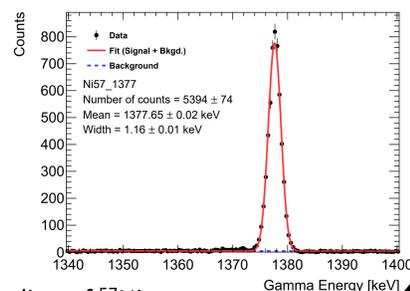
➤ Right: Example of the desired gamma decay line of  $^{57}\text{Ni}$ .
