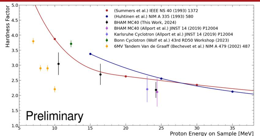
A summary of the three hardness factor measurements from this study, along with other experimental data in the energy range. The theoretical curves by Summers and Huhtinen have been interpolated from the discrete predictions.
