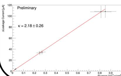
An example of the change in leakage current versus fluence points (27 MeV). The uncertainty on  $\kappa$  is dominated by the current scaling extrapolation and the fluence uncertainty (cross-section measurements and our understanding of the HPGe detector efficiency).
