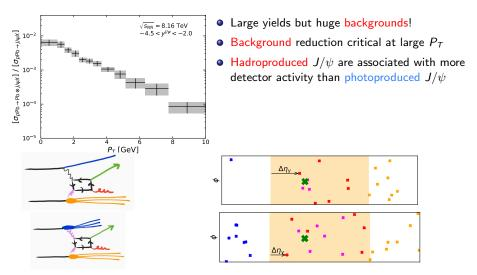
3 background-reduction techniques based on different detector acceptances: central Δη<sub>γ</sub>: distance in rapidity between main detector on photon-going side and closet particle activity
