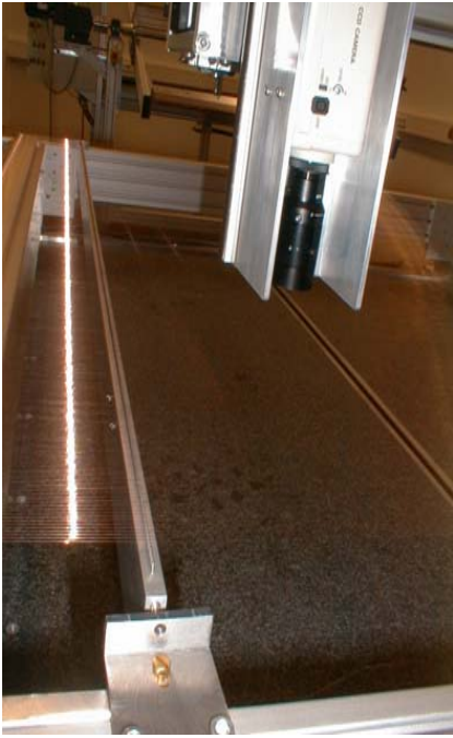
Wire grid assembly and inspection
