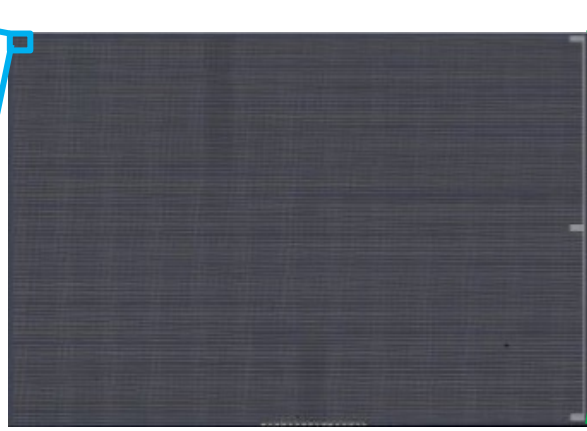
SiPM: 12x8 mm (NUV-HD-Cryo SiPMs from FBK)
