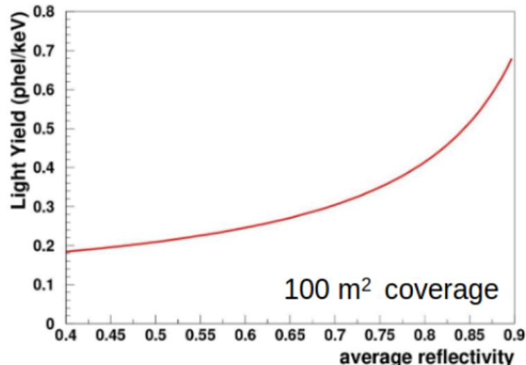
The most relevant parameters for the LY are the **active coverage with SiPM** and the **reflectivity of internal surfaces**. For  $R > 70\%$  there is a rapid increase in the LY.
