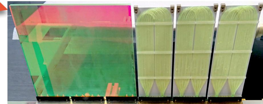
Light detectors digitized when a waveform from 1 ArCLight or 3 LCMs surpasses a self-trigger threshold (Or digitized when a beam signal is received)
