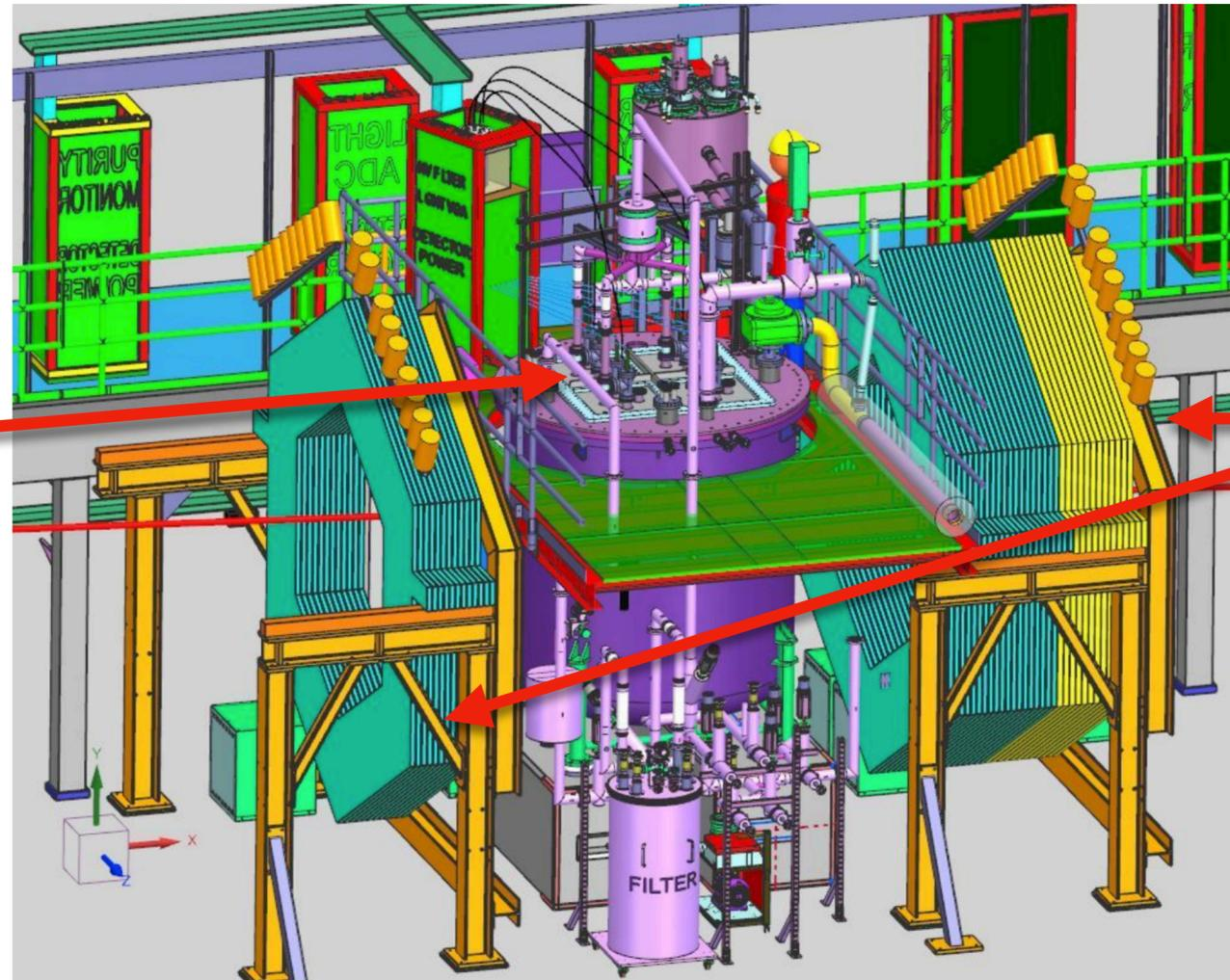
Four  $1.2 \times 0.6 \times 0.6 \text{ m}^3$  LArTPC modules in a 2x2 array (smaller than the ND-LAr modules)
