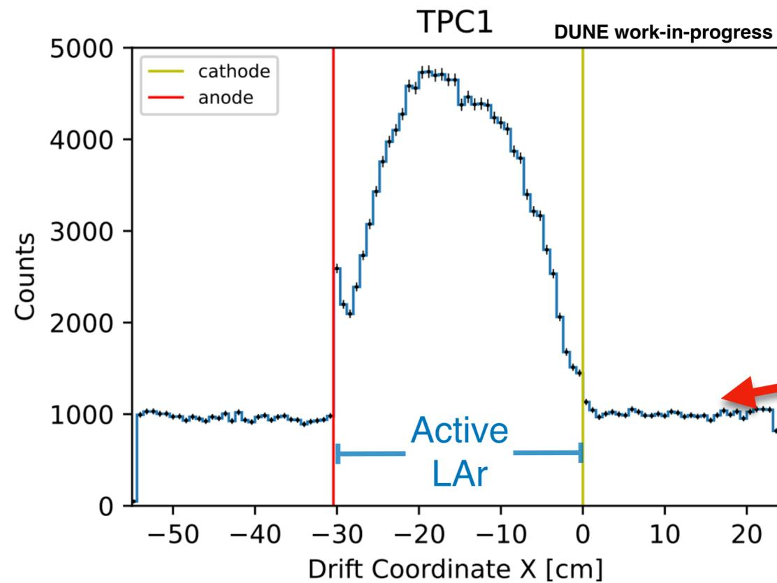
The extended window allows us to estimate purity using the flat sidebands
