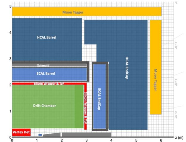
**ALLEGRO detector layout with ECAL as the core housed inside the solenoid**
