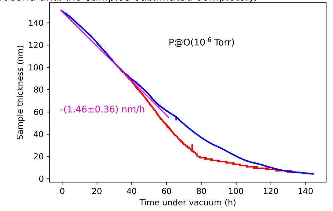
As illustrated in the figure above, the samples demonstrate a clear trend of sublimated when subjected to vacuum conditions. Additionally, by comparison with the figure below, it is evident that the evaporation rate is pressure-dependent,
