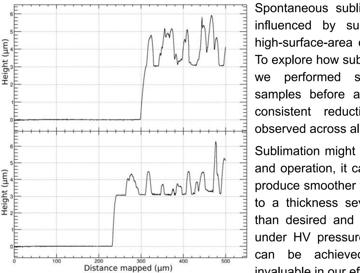
Spontaneous sublimation is a process that can be influenced by surface area, potentially impacting high-surface-area crystal growths on thick pTP films. To explore how sublimation affects surface roughness, we performed surface profilometry on multiple samples before and after exposure to vacuum. A consistent reduction in surface roughness was observed across all tested samples.
