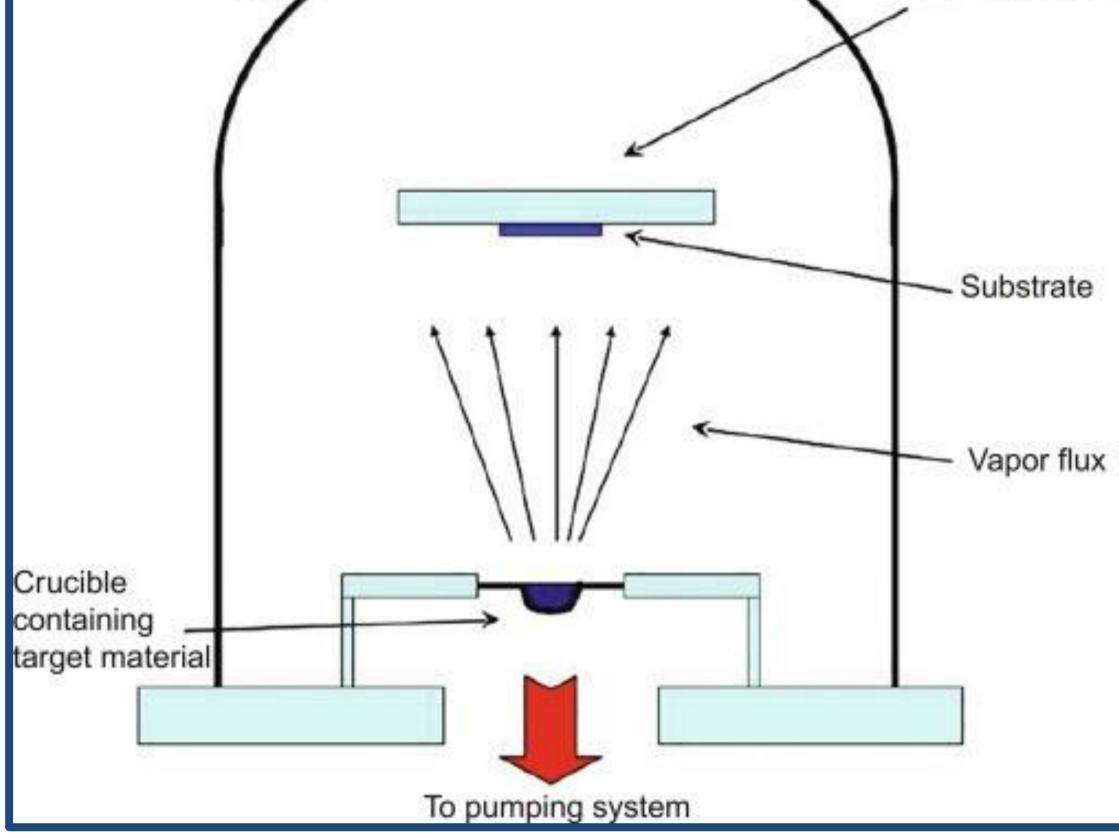
employed method for fabricating thin films. In this process, the material intended for deposition is heated in a crucible within a vacuum chamber, causing it to and sublimate generate a molecular flux. The low pressure environment (10<sup>-6</sup> Torr) ensures a high mean free path for the molecules, allowing them to travel directly to the substrate without collisions. Upon reaching the cooler substrate surface, the molecules condense and form a well-adhered thin film.
