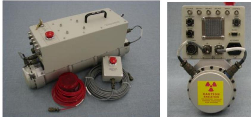
Commercial Thermo Fisher MP-320 Deuterium-Deuterium Generator (DDG), which produces monoenergetic 2.45 MeV neutrons with a flux of up to  $10^6$  neutrons/second.
