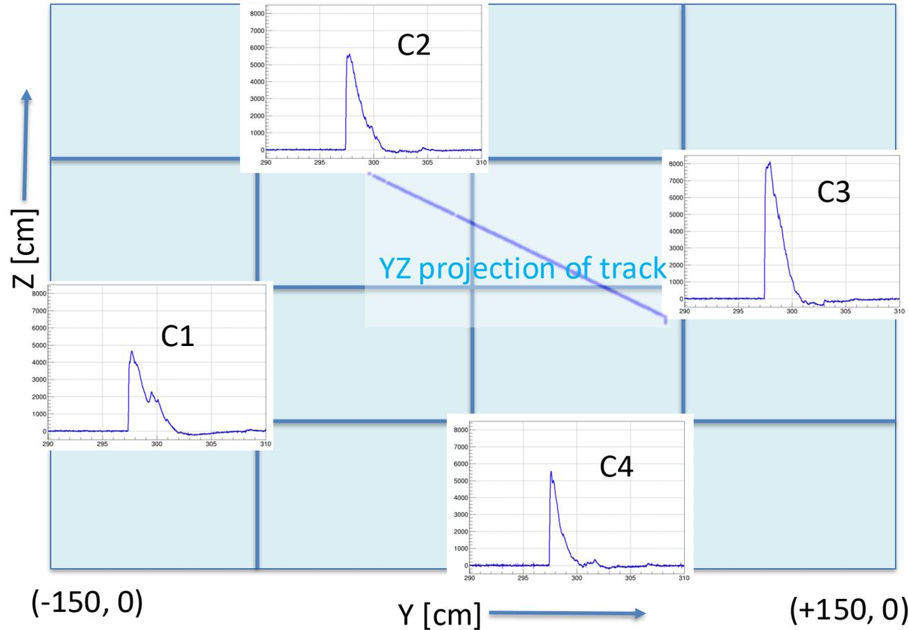
The grids on the left shows the cathode frame and the waveforms for the 4 X-ARAPUCA channels at corresponding location.
