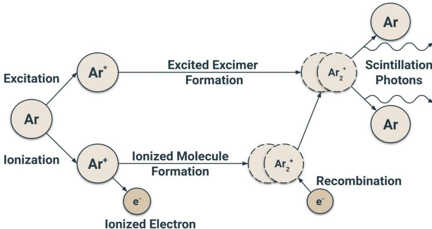
Fig: Mechanism of scintillation light production in Ar.
