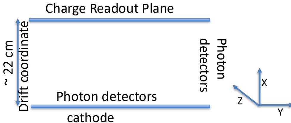
Drift distance ~22cm; length ~3m and width ~3m
