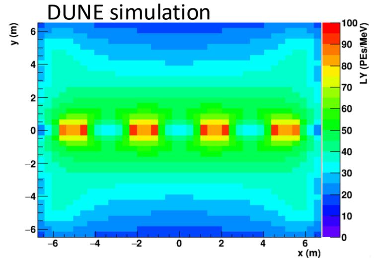
Fig: Map of the light yield (LY) in the central (x, y) transverse plane at  $z = 0$  for the reference configuration.
