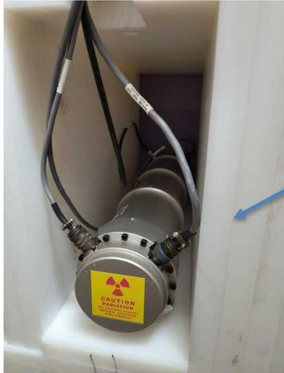
Polyethylene shielding enclosing PNS
