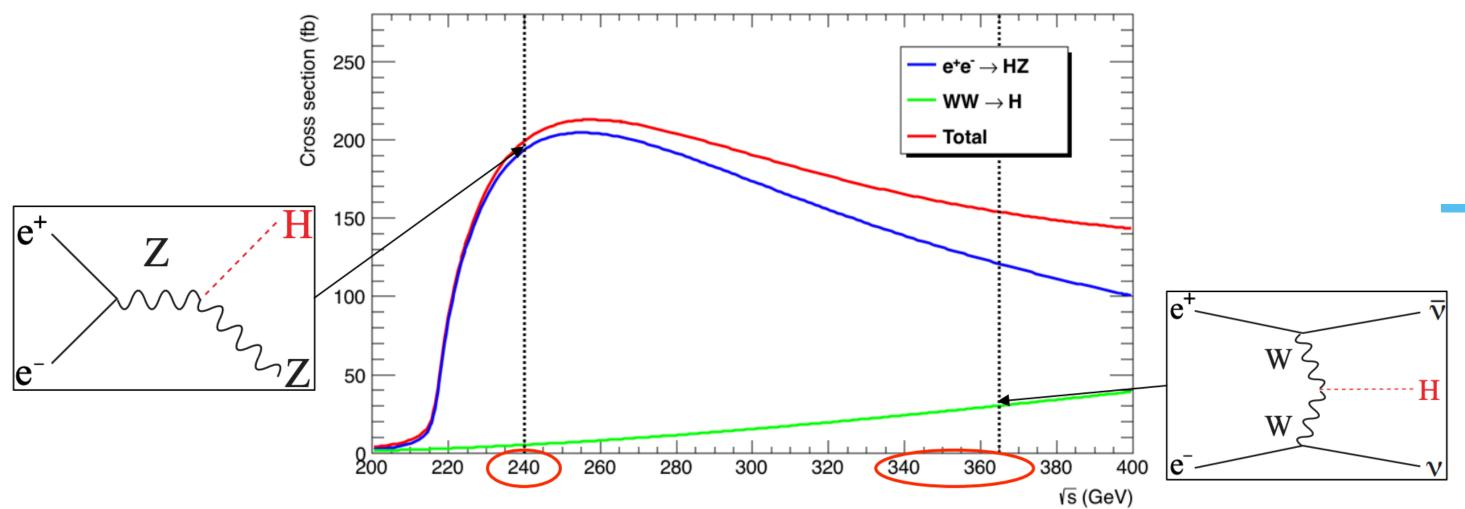
Fundamental properties: model-independent ZH cross section, mass, width, self-coupling, CP **Brs/Couplings:** ZZ&WW, Hadrons (bb,cc,ss), Leptons ( $\tau\tau$ ), Rare ( $\gamma\gamma$ , Z $\gamma$ , $\mu\mu$ ), Exotic (BSM/invisible),
