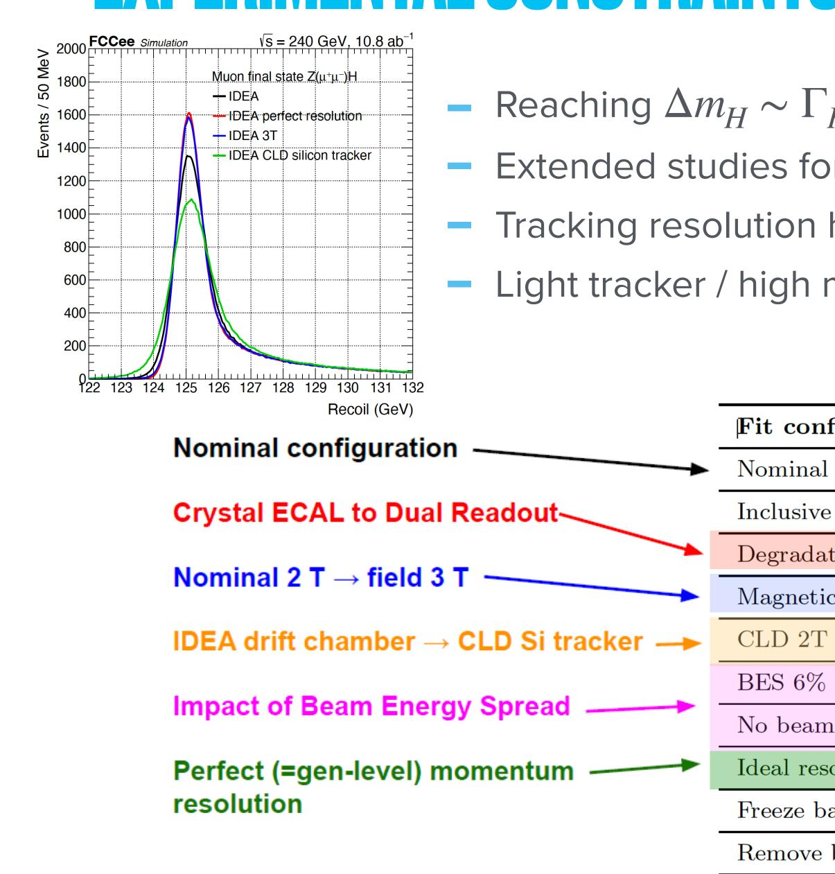
Reaching  $\Delta m_H \sim \Gamma_H \sim 4$  MeV requires outstanding detector performance Extended studies for key detector effects: feedback to detector design Tracking resolution highly impacts m<sub>H</sub> precision Light tracker / high magnetic field preferable
