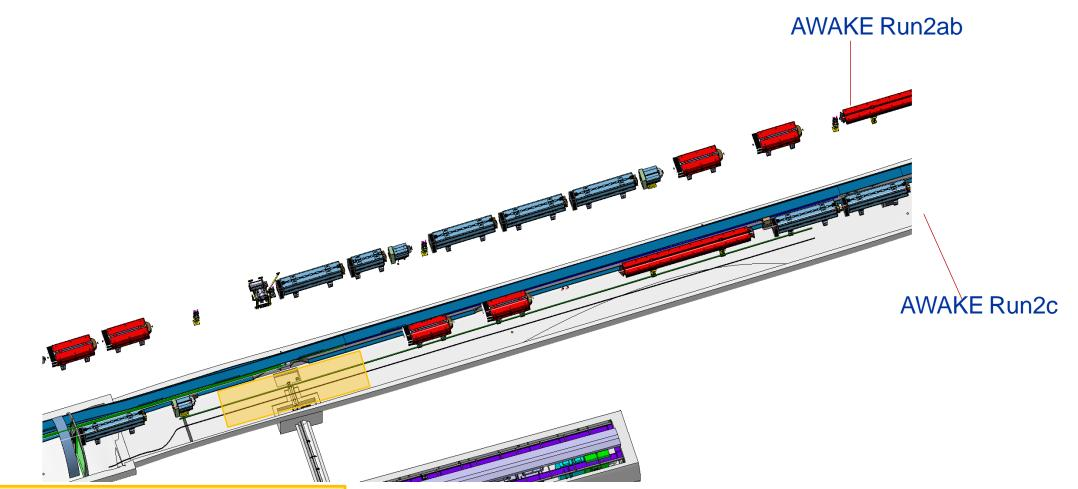
Laser Merging Mirror Equipment  $\rightarrow$  move 35m downstream relative to Run2ab position. Proton beam magnets  $\rightarrow$  relocate to support the Run2c plasma cell1 location and avoid conflicts with infrastructure, e.g. doors, in the tunnel.
