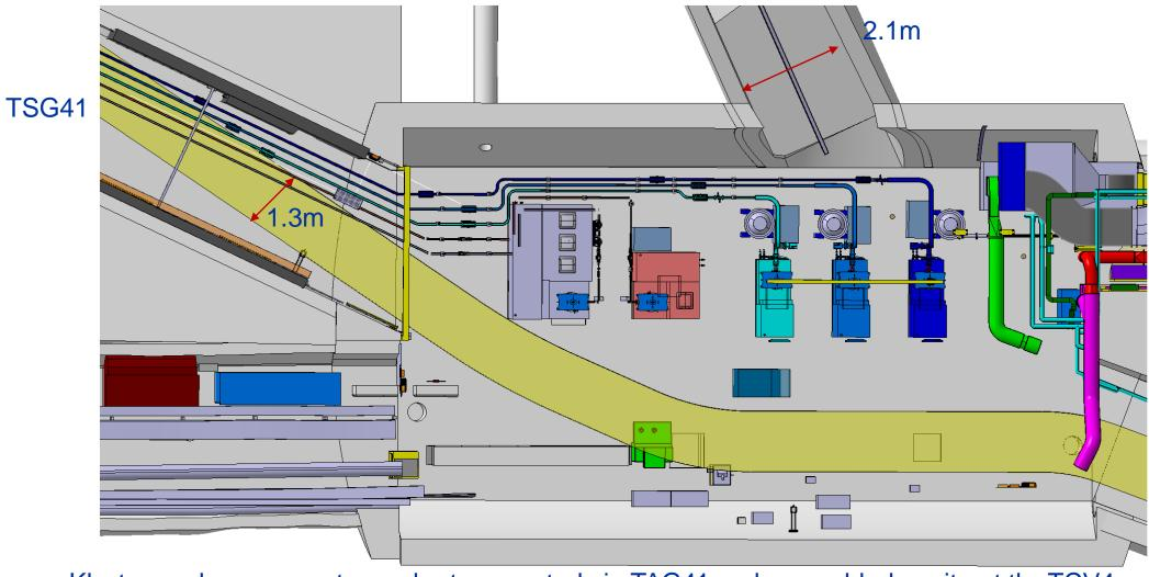
Klystron subcomponents can be transported via TAG41 and assembled onsite at the TCV4.
