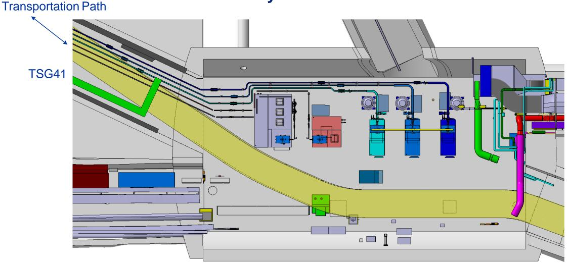
Double spaces required for Run2c (additional) klystrons  $\rightarrow$  TCV4 allows a perfect location with optimum waveguide length.
