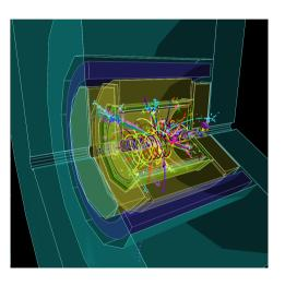
The International Large Detector (ILD) is a detector concept for both Linear and Circular e+e- Colliders. Dedicated CC design version implemented, full simulation studies ongoing...
