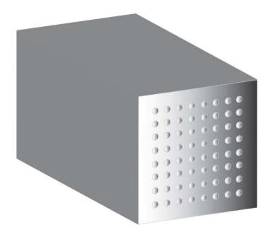
Scintillating fibers are bundled and terminated at a photodetector behind the calorimeter.
