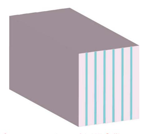
Scintillating plates are readout with WLS fibers and the light is
