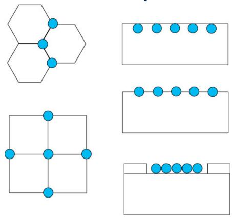
There are infinite possibilities but we must consider the relevant scaling factors (e.g. Moliere radius in transverse and radiation/interaction length in longitudinal directions) and weight them against practical limits.
