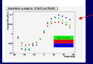
Difference in collected light is plot vs. beam incidence angle
