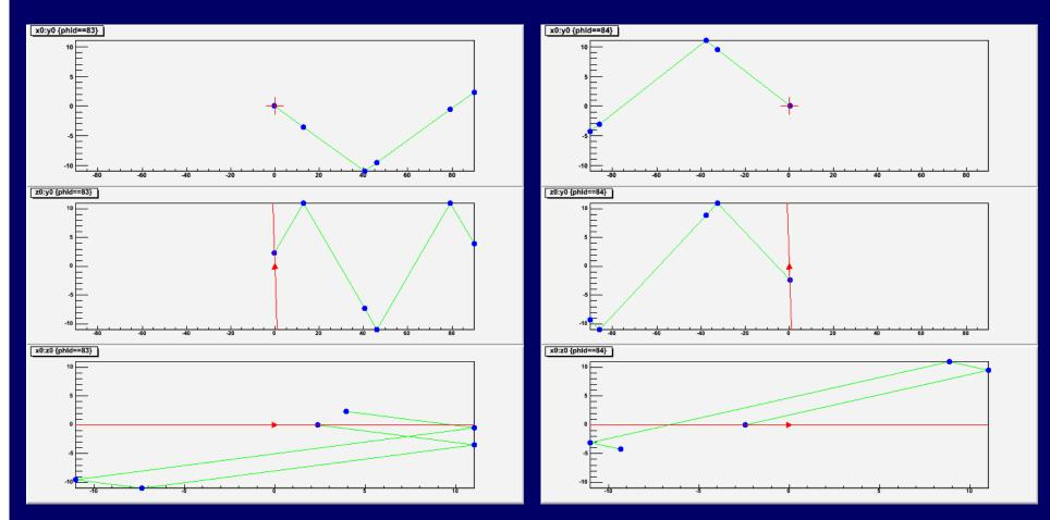
Cerenkov photon exiting the crystal on the RIGHT side after 4 reflections Cerenkov photon exiting the crystal on the LEFT side after 3 reflections
