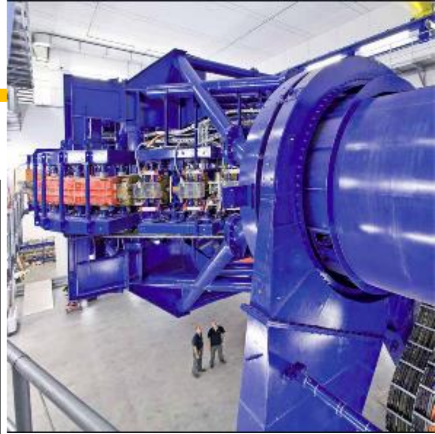
HIT carbon gantry
