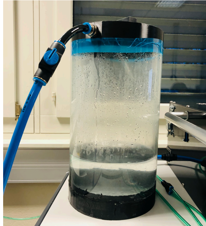
Cooling water tank
