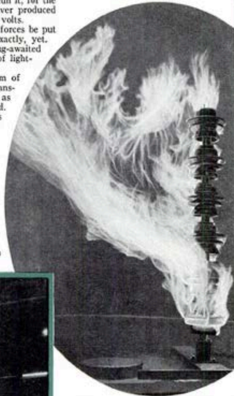
This is not lightning, but a discharge of laboratory electricity leaping from insulators. It shows why extraordinary apparatus is required in harnessing 18,000,000 volts.
