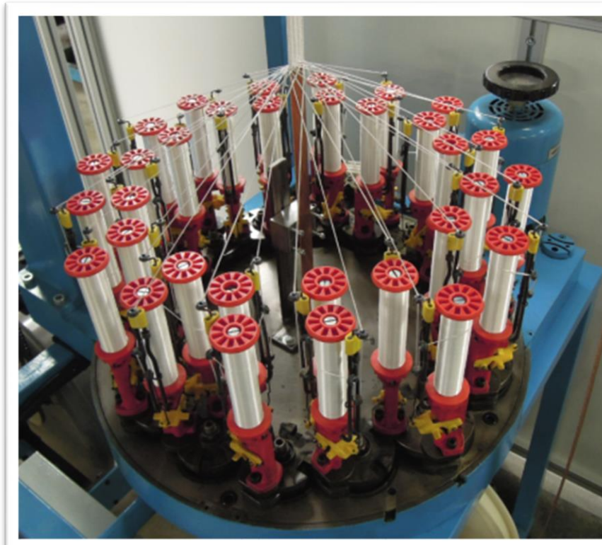
Fiber glass insulation for \text{Nb}_3\text{Sn}
