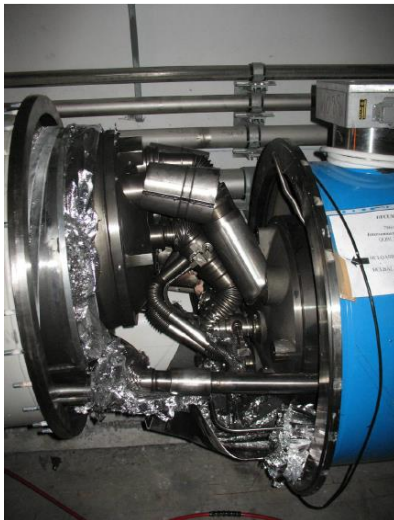
Result of the chain of events triggered by a quench in an LHC bus-bar
