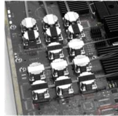
Figure 2. MiniPOD™ Transmitter and Receiver flat ribbon cable modules in a tiled arrangement example.
