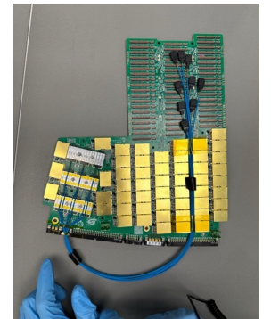
First 2 of most complex HGTD PEB prototypes produced and under test
