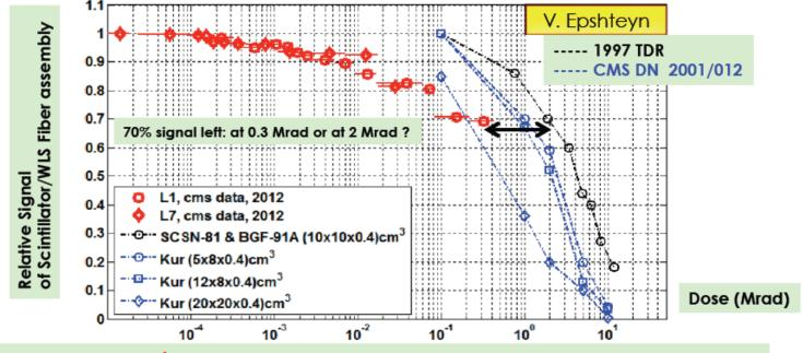
For CMS data at 22 fb<sup>-1</sup> (Red points), dose is calculated using FLUKA simulation (M. Guthoff)
