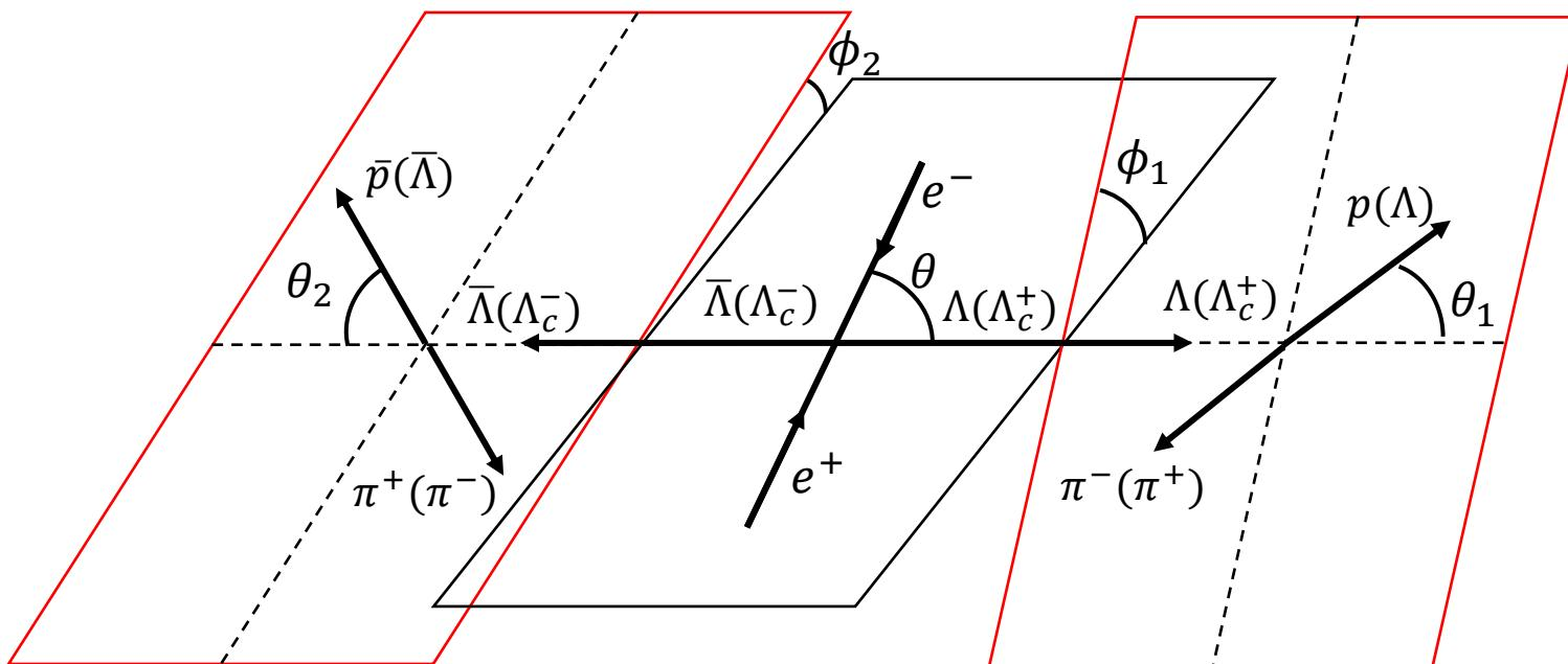
A schematic representation of the kinematics of the two-step process of annihilation of an electron-positron pair into a pair of heavy baryons decaying into a baryon-meson pair.
