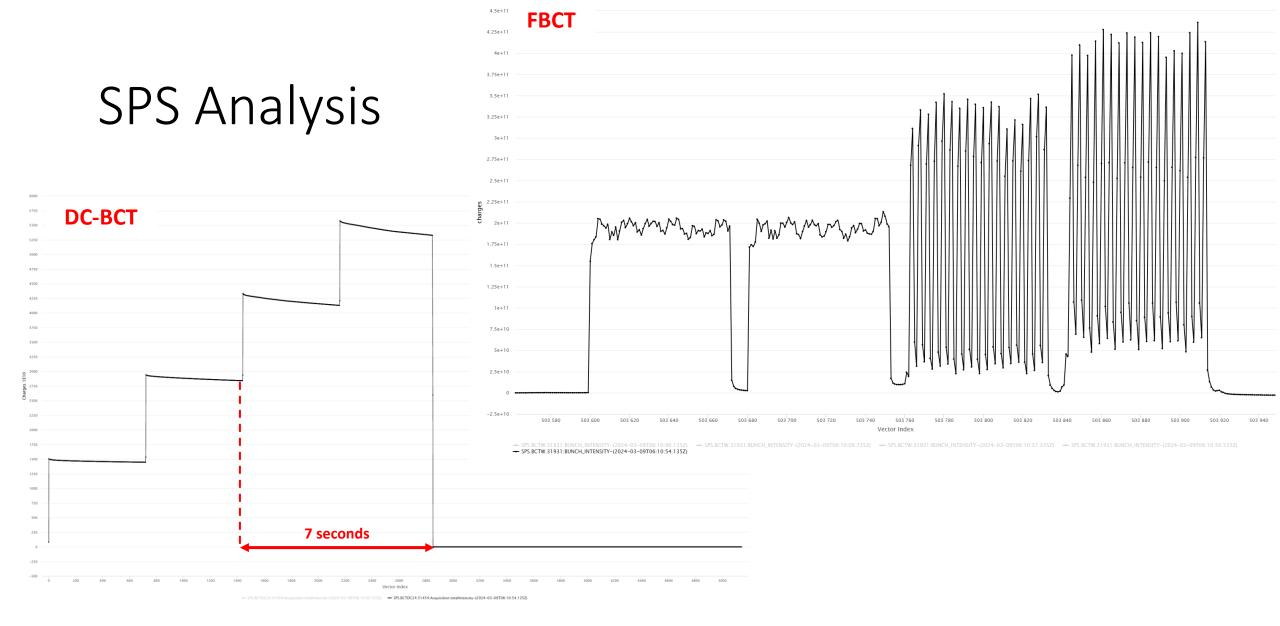
2b+2e beam with 36b of >4e11 was injected for last two injections and circulated for ~7 seconds until beam was dumped
