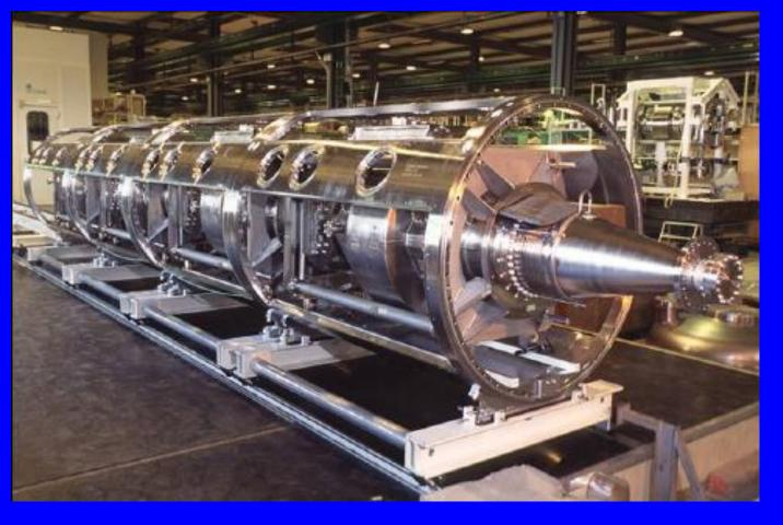
8 radiofrequency (RF) cavities for each beam, installed in groups of 4 in cryomodules, accelerate the beams
