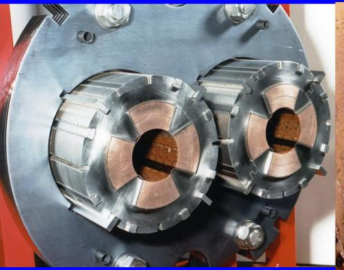
quadrupole magnets focus the beams
