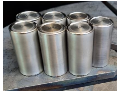
Capsules after EB welding
