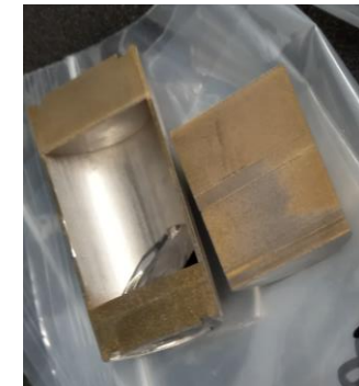
Single failed UT capsule fell apart when cut open
