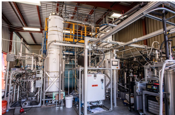
Offsite Kr removal of 10t of LXe at SLAC
