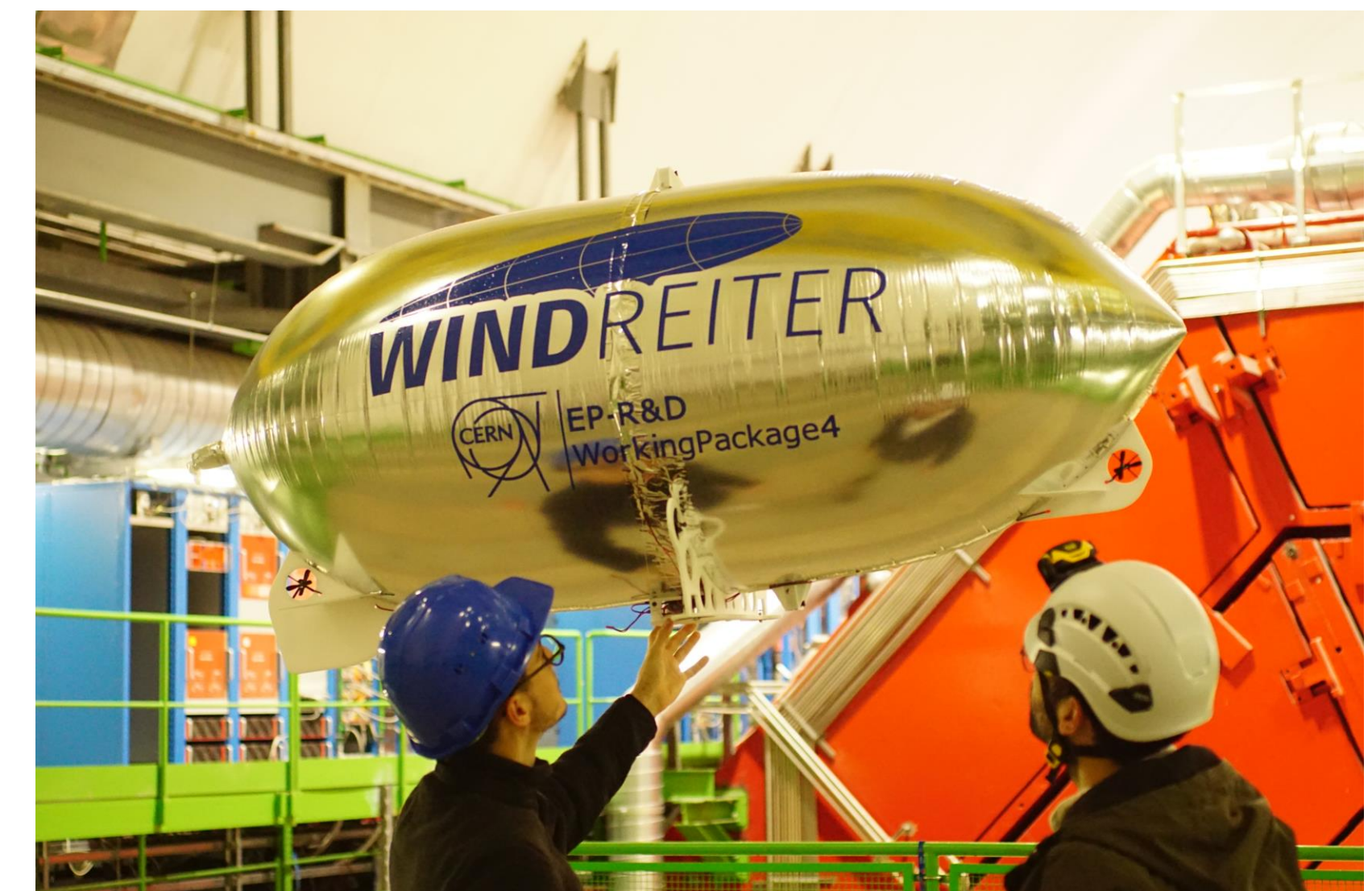
Test of the first teleoperated blimp prototype in the ALICE Cavern.
