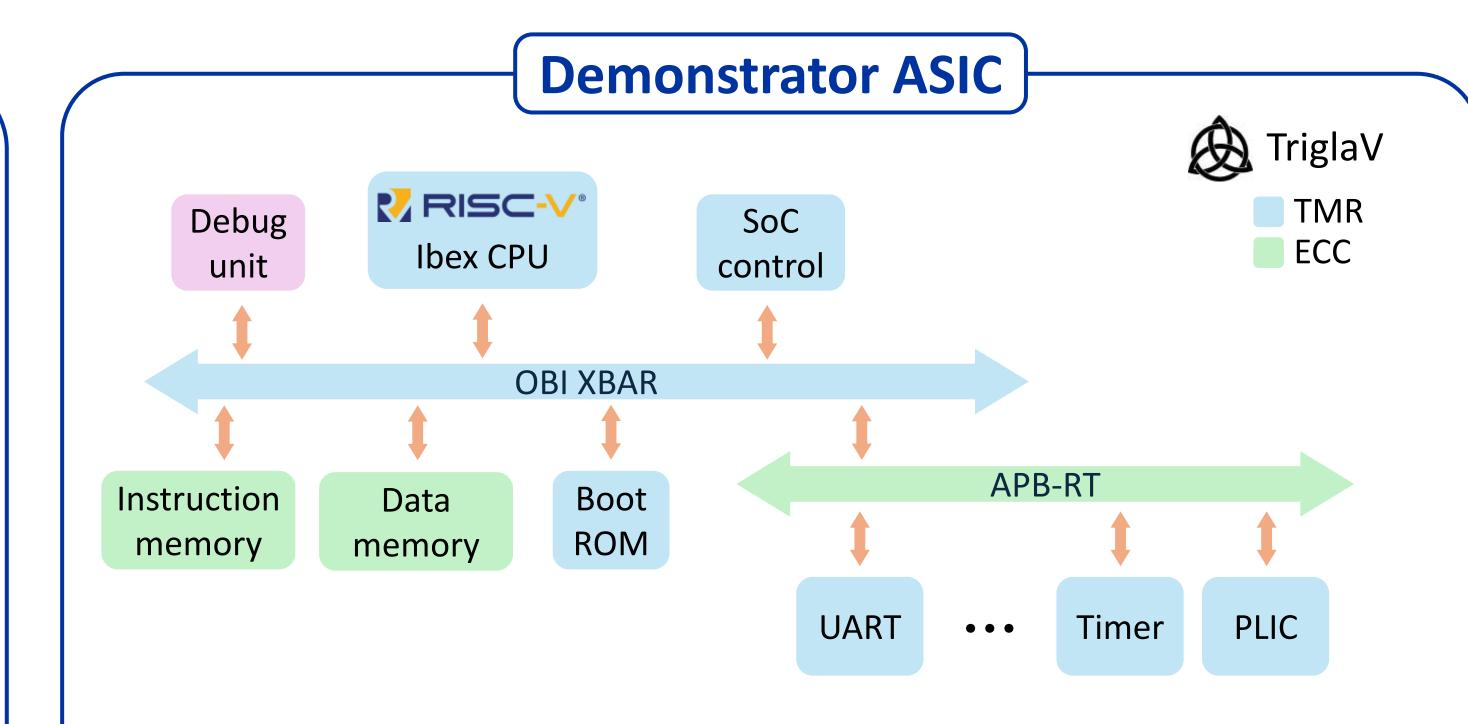
To validate this toolset and test the radiation performance of the resulting design, a demonstrator chip is being developed in a commercial 28nm bulk CMOS technology. This SoC is generated using the SOCRATES platform and it's based around Ibex, an open-source RISC-V processor core. A minimum set of peripherals is included, while maintaining a focus on introducing observability and testability features to evaluate the radiation tolerance of the design under irradiation testing.
