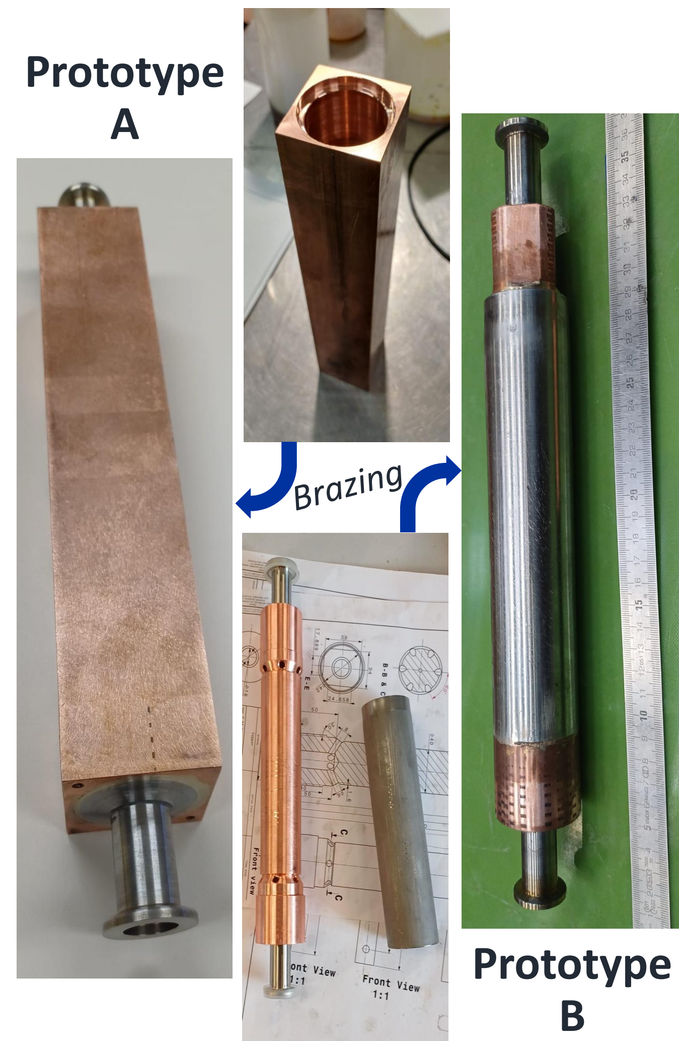
Fig. 3 - Photographic images of heat interceptors before and after assembly.
