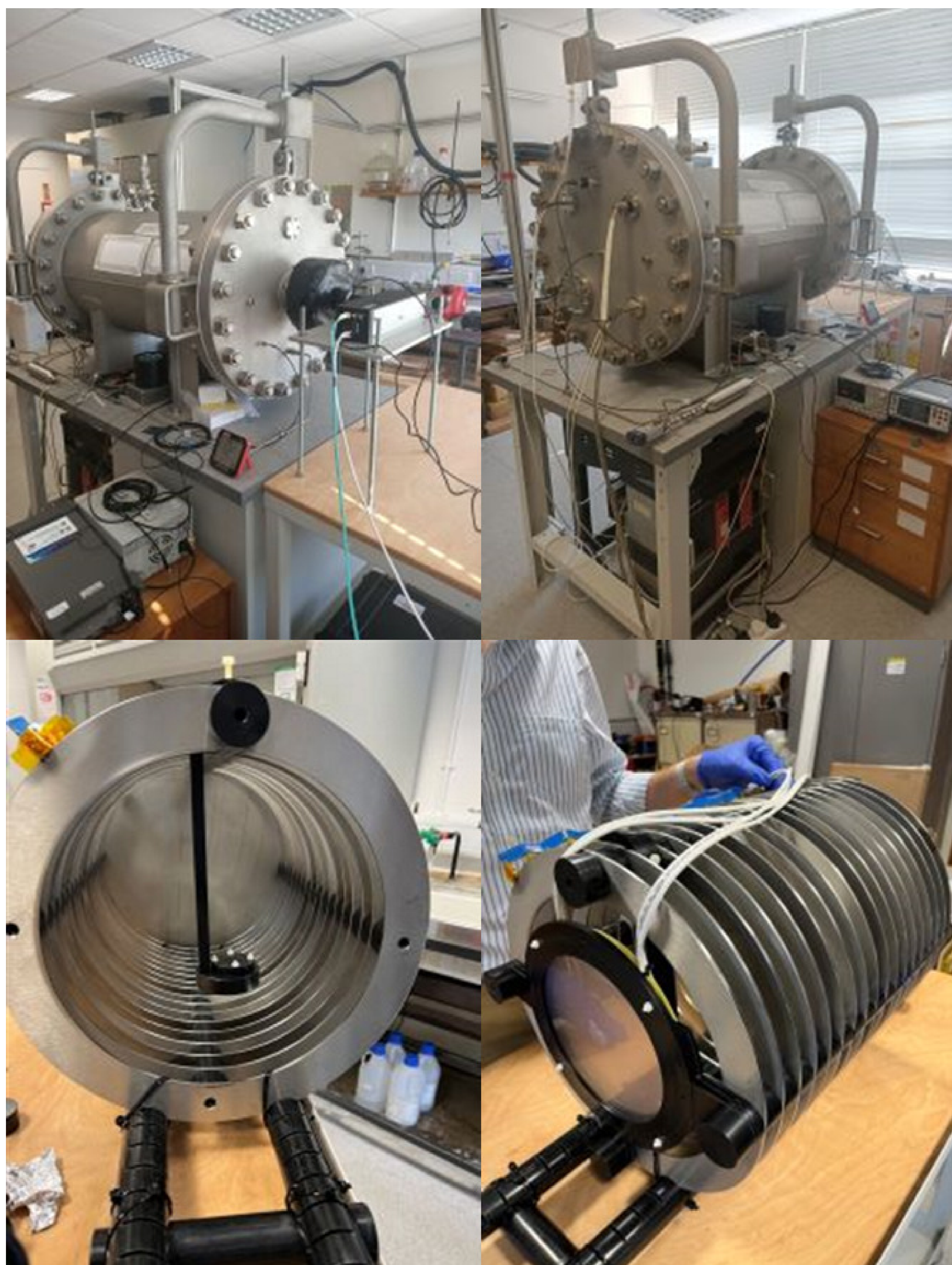
Fig. 1: The WarTPC pressure vessel shortly after being moved into the lab (top left and right), the current TPC setup (bottom left), and the pressure vessel including the sensor feedthroughs and gas system (bottom right).
