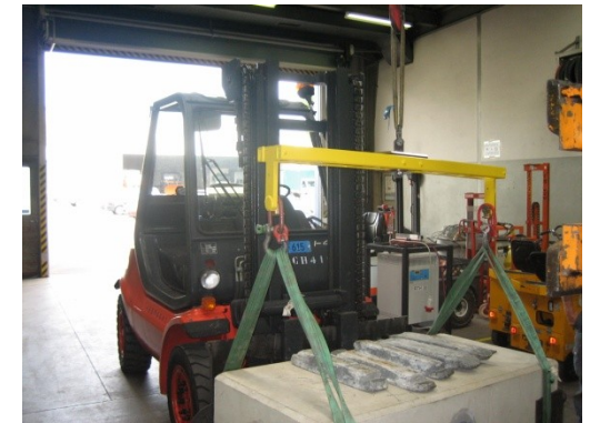
Spreader beam load test
