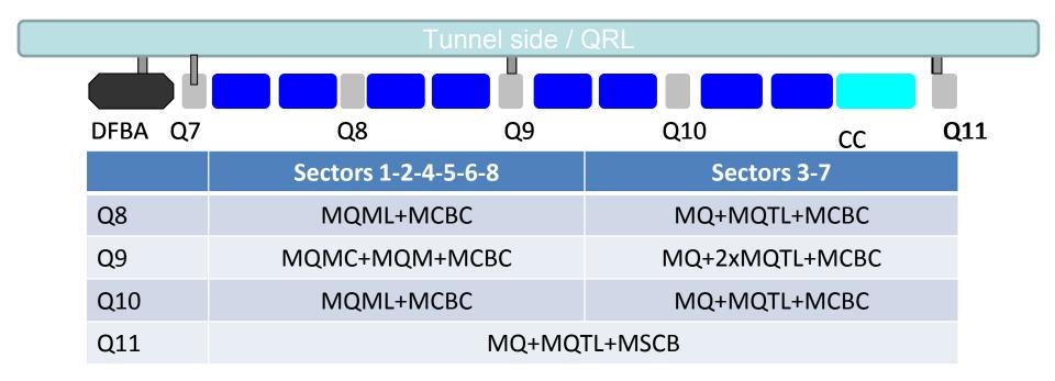
Q8-Q10-Q11 are 6620 mm long, Q9 is 8020 mm long, all magnets @ 1.9 K
