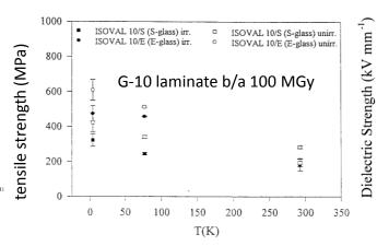
source: workshop on advanced materials for high precision detectors, CERN, 1994 Tests done according to IEC 544 with  $\gamma$
