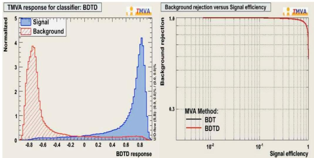
TMVA results in 5% efficiency for s-tagging with  $10^3$  b-jet rejection.
