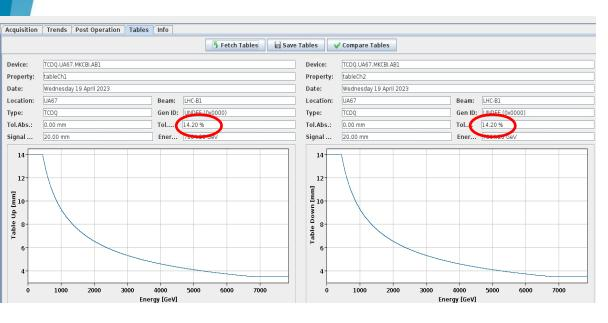
Due to criticality of correct positioning of TCDQ to ensure the protection of the machine in the rare event of an asynchronous beam dump → additional fully independent verification of TCDQ position with respect to the energy done by the Beam Energy Tracking System (BETS) using an additional potentiometer
