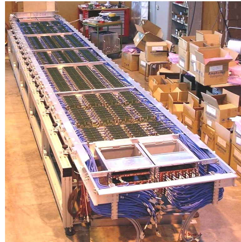
Supermodule (8 m, \sim 8000 TOF channels)
