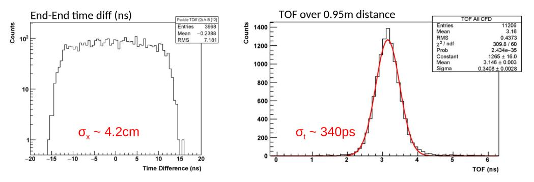
fast sampling with custom-made readout board, based on the DRS-4 ASIC: <400ps timing resolution achieved
