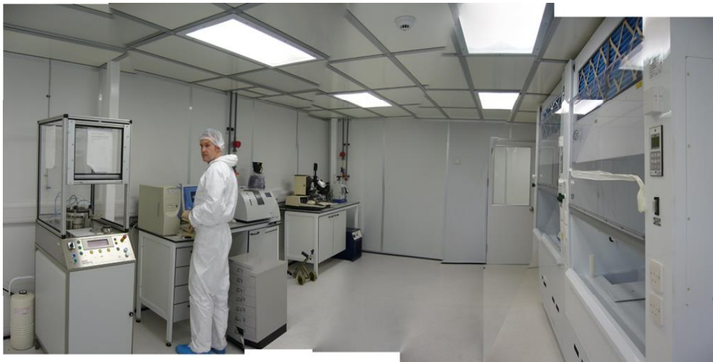
Class 10 000 area (Bio, Photochemical, MEMS, Photolith cabinets)
