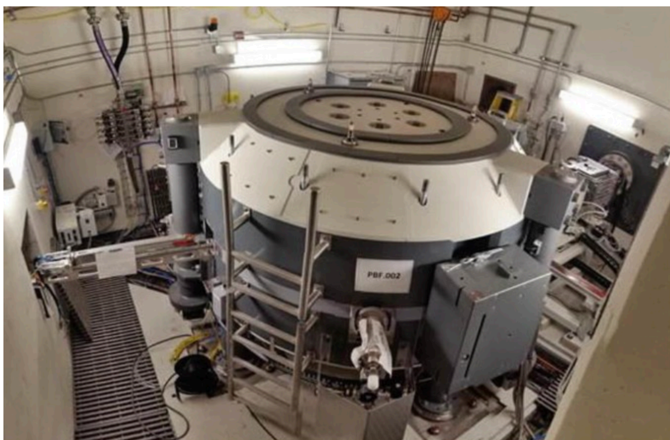
IBA Proteus one superconducting cyclotron (230 MeV protons)
