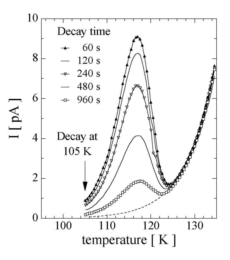
The peak temperature is not a terribly precise way to extract the activation energy of the traps - can instead perform measurements at different times and temperatures to extract true activation energy
