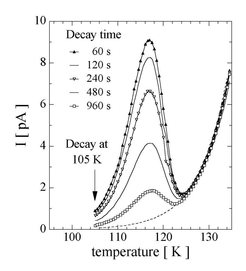
The peak temperature is not a terribly precise way to extract the activation energy of the traps - can instead perform measurements at different times and temperatures to extract true activation energy
