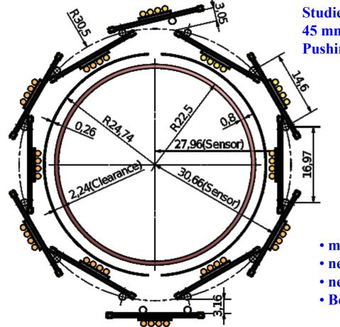
Studies are ongoing to asses safe beam pipe radius. 45 mm diameter seems doable. Pushing for Beam Pipe installation in LS1 2013
