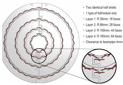
**Total** Number of Pixel modules: 1.888 Number of Pixel: 124 M Sensor Area: 2 m<sup>2</sup> of Pixel detector
