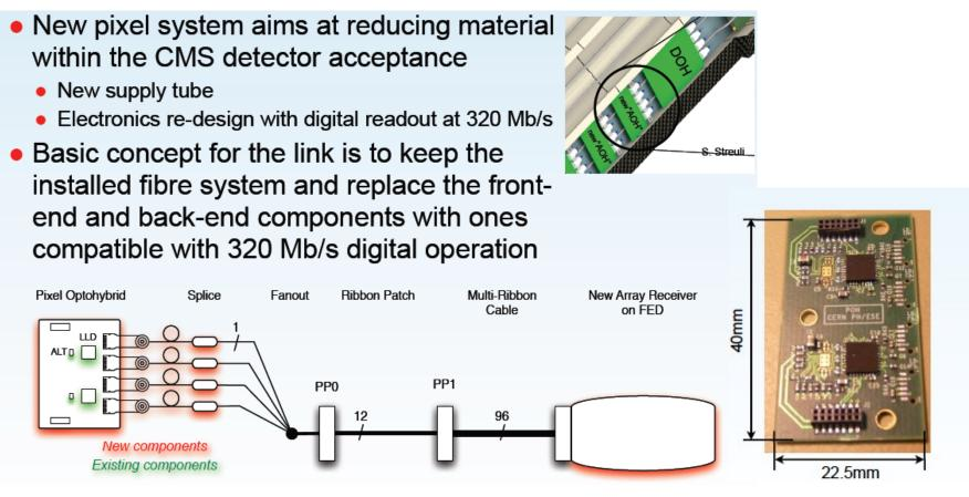
Activity advancing well at CERN. First Pixel Opto Hybrid (POH) prototypes with new laser available for evaluation
