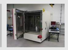
Environmental test facility is used to evaluate pump performance at various ambient temperatures and humidities.
